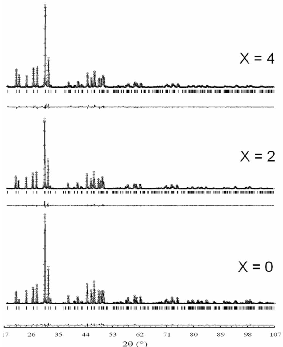
**Figure 1.** Experimental and calculated X-ray diffraction patterns, and their difference of  $\text{Sr}_{10}(\text{PO}_4)_6\text{O}$ ,  $\text{Sr}_8\text{La}_2(\text{PO}_4)_4(\text{SiO}_4)_2\text{O}$  and  $\text{Sr}_6\text{La}_4(\text{PO}_4)_2(\text{SiO}_4)_4\text{O}$ .
