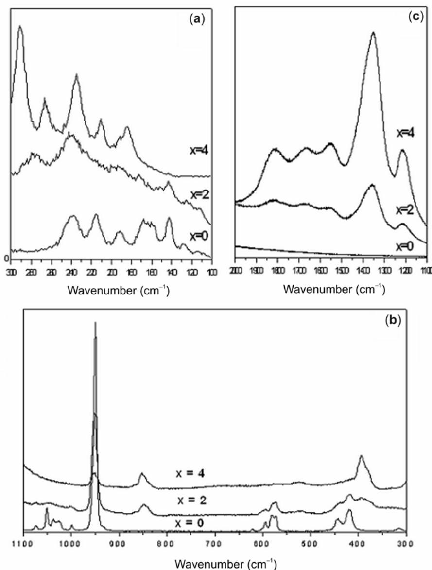
**Figure 2.** Raman spectra of  $\text{Sr}_{10-x}\text{La}_x(\text{PO}_4)_{6-x}(\text{SiO}_4)_x\text{O}$  samples: Spectral ranges were in (a)  $100\text{--}300\text{ cm}^{-1}$ , (b)  $300\text{--}1100\text{ cm}^{-1}$  and (c)  $1100\text{--}2000\text{ cm}^{-1}$ .
